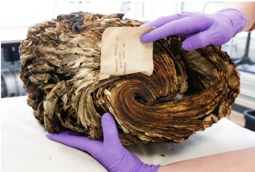
Figure 2: Fire damaged 19th-century legal documents in parchment © National Archives of Ireland. Reproduced with the kind permission of the Director of the National Archives.
