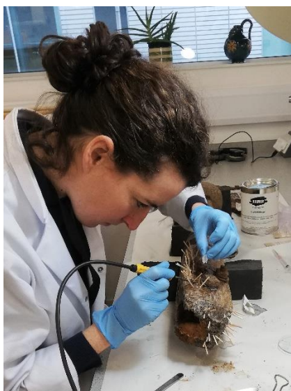
Figure 4: Application of Cyclododecane onto wood surface © Róisín Beirne.
